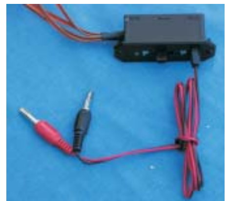
The 12 amp heavy duty switch harness with the external charging lead plugged in. A green LED indicates power is on.
