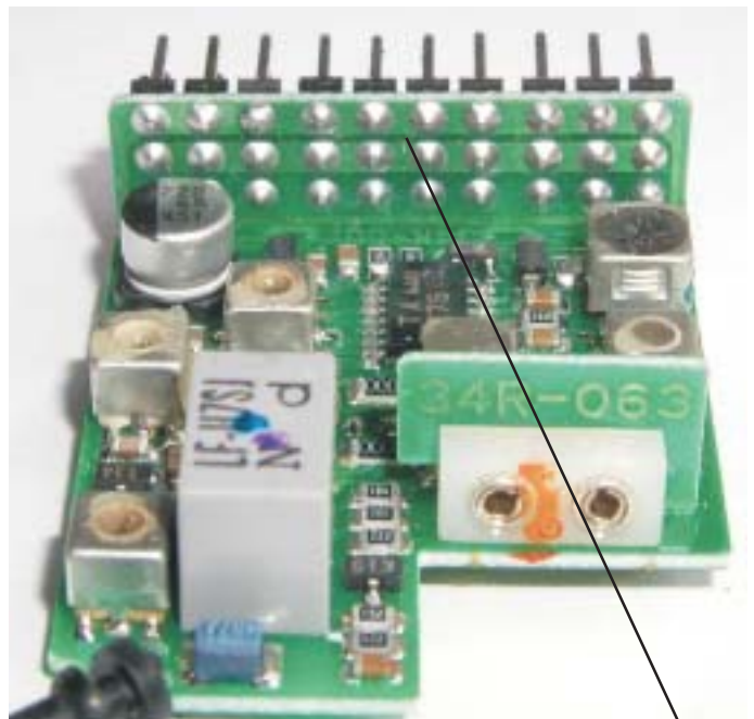
In a typical receiver, the positive and negative servo power is distributed to each servo on these power bus PC lands from the battery socket pins.
