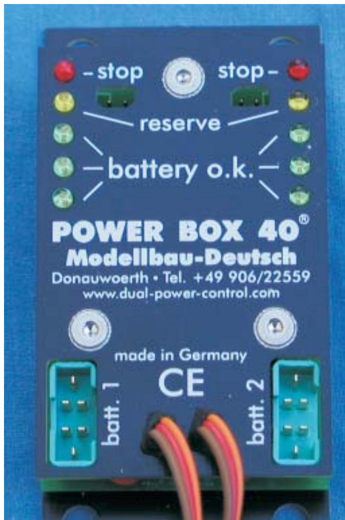
The basic Power Box 40. Two battery supply to RX and voltage indication for four or five cell battery packs.
