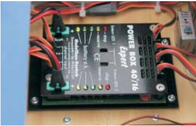
A Power Box 40/16 installed in Steve Annett's turbine powered Eurosport handles the power requirements on this large and heavy model. Pictured below is Steve prepping the model before a flight at Temora.
